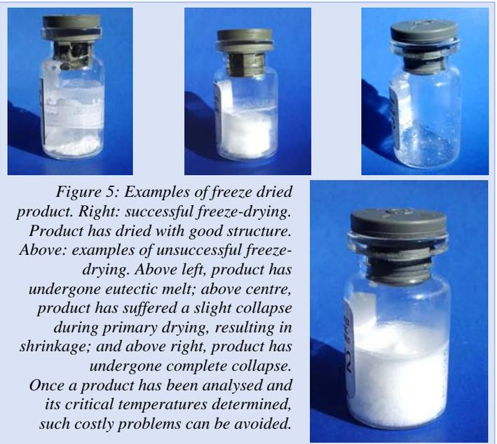
Figure 5: Examples of freeze dried product. Right: successful freeze-drying. Product has dried with good structure. Above: examples of unsuccessful freeze-drying. Above left, product has undergone eutectic melt; above centre, product has suffered a slight collapse during primary drying, resulting in shrinkage; and above right, product has undergone complete collapse. Once a product has been analysed and its critical temperatures determined, such costly problems can be avoided.
