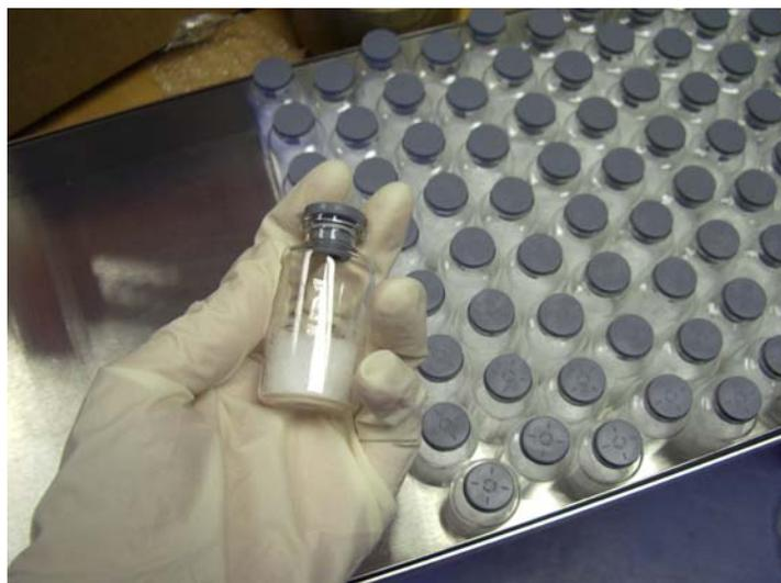
Figure 2: Freeze drying in vials
