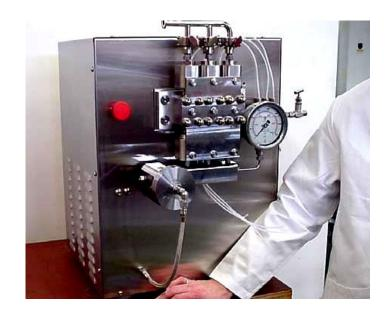
The C55 is electrically-powered, with a triplex pump designed for quiet operation and high throughput.
