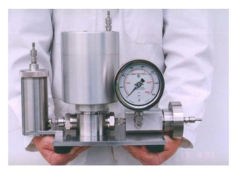
Pressures of up to 30,000 psi enable the EmulsiFlex C5 to process the toughest samples. With a footprint of  $43 \times 17 \times 31$  cm and weighing only 25kg, the C5 is compact enough to fit onto the most overcrowded lab bench without compromising power or performance.
